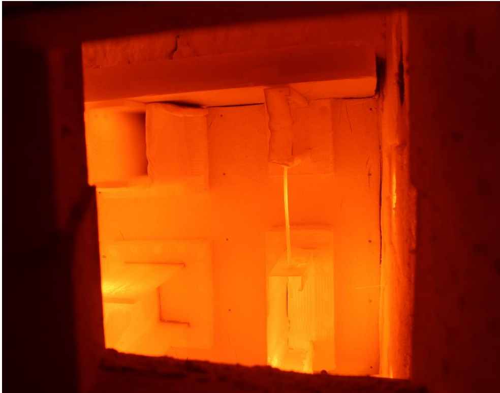
Figure 21 – Exposed face at 120 minutes
