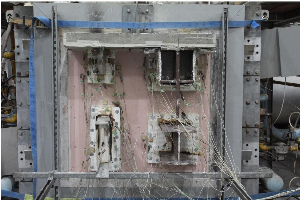
Figure 20 – Unexposed face at 120 minutes
