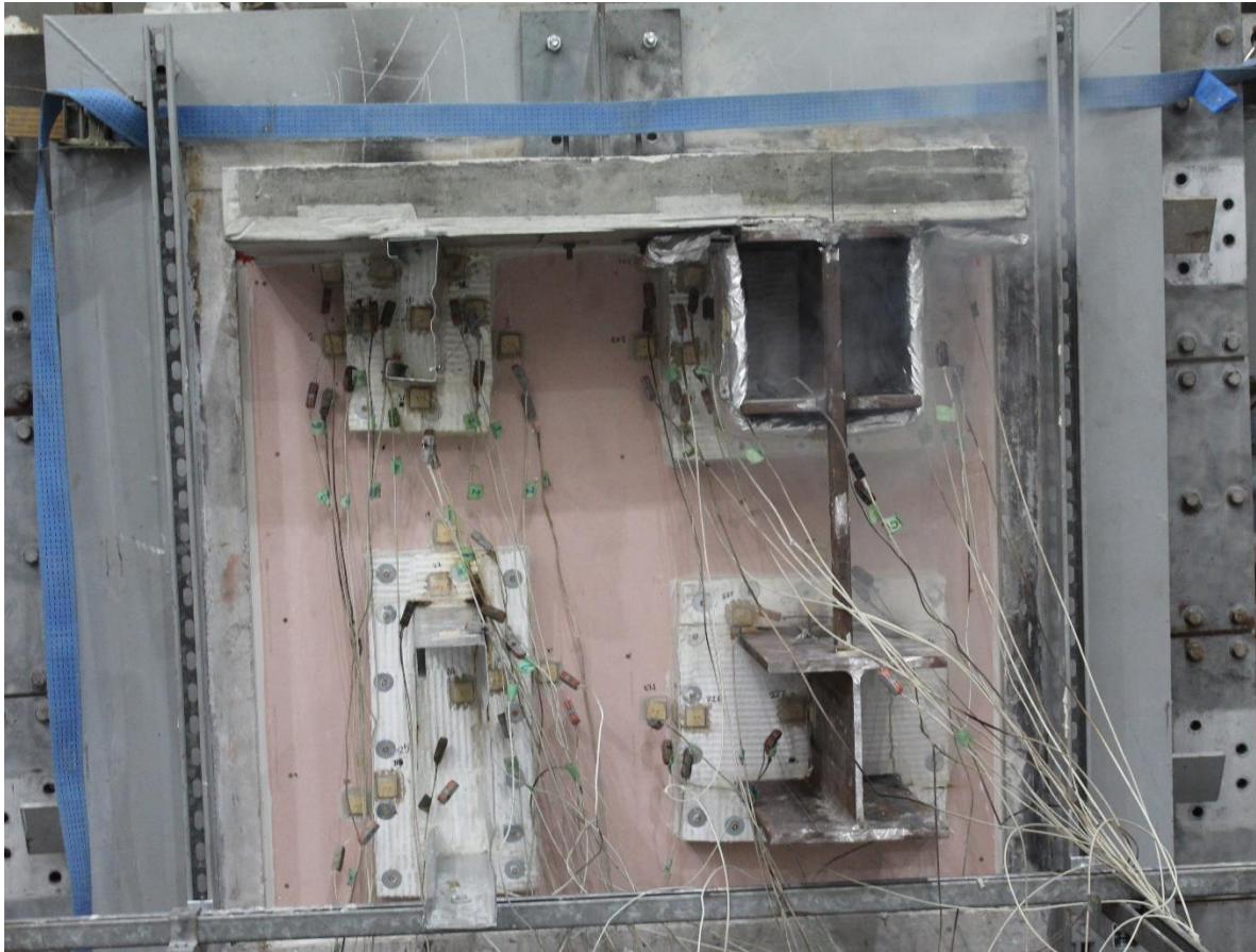
Figure 15 – Unexposed face at 60 minutes
