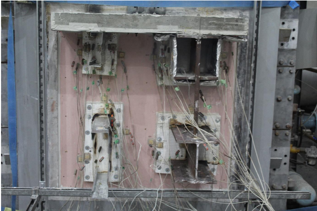
Figure 19 – Unexposed face at 105 minutes
