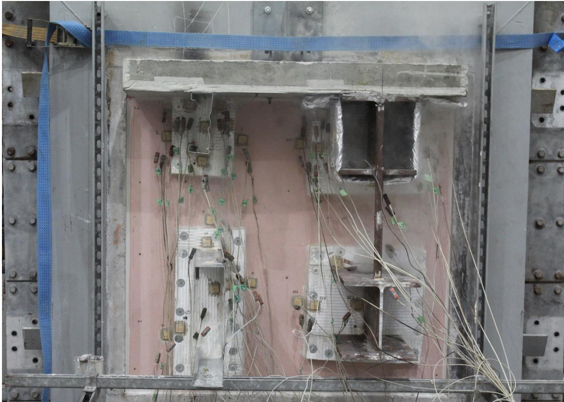
Figure 11 – Unexposed face at 30 minutes
