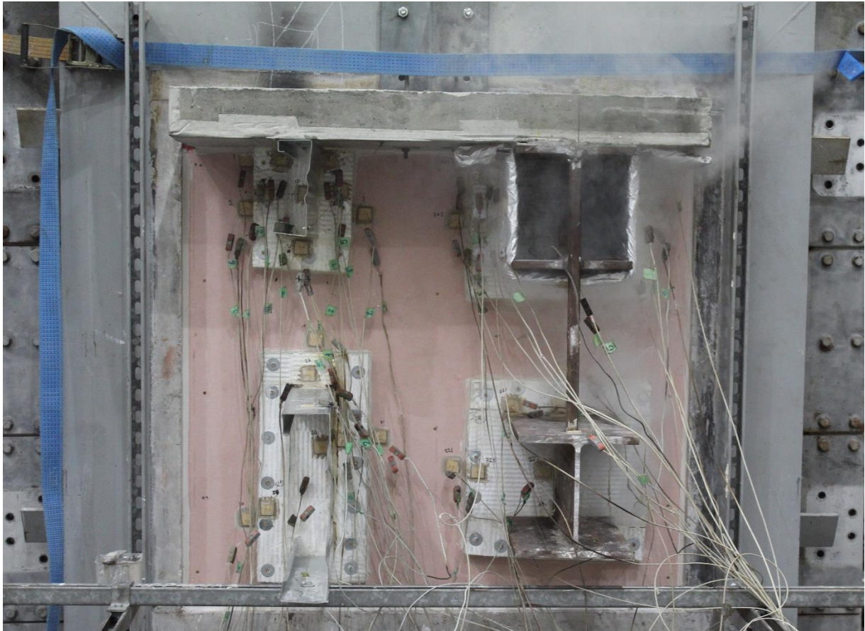
Figure 13 – Unexposed face at 45 minutes
